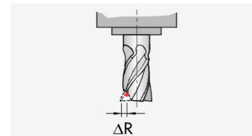
Tool radius measurement, detection of tooth breakage
