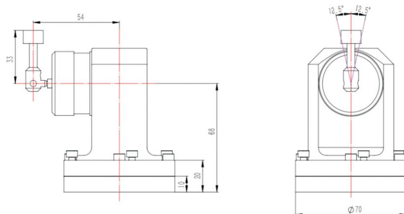
The SPTS series tool setter composed by a photoelectric switch, a with high hardness and wear resistance contact, a signal transmission interface. the photoelectric switch is key parts, When the sensor beam is interrupted, a trigger signal will be sent out and transmitted to the NC system through the interface device to identify, calculate, compensate and access the tool length
