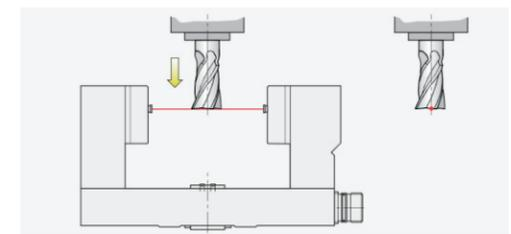
Detection of tool breakage
